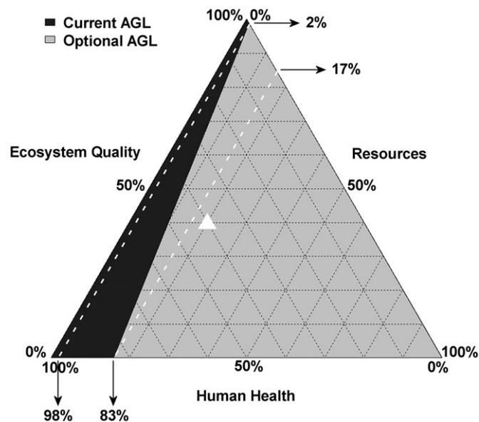
Fig. 4. Mixing triangle results of the two AGL systems, using the EI99 method.
