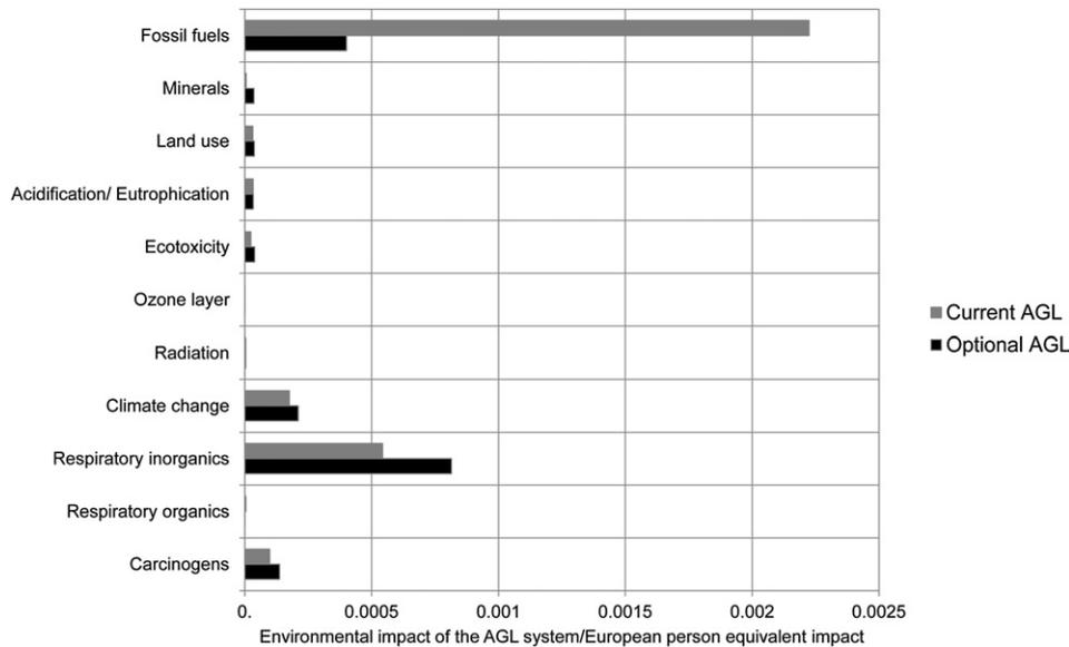
Fig. 3. LCIA normalization results of the two AGL systems, using the EI99 method (adapted from Simões et al., 2010).
