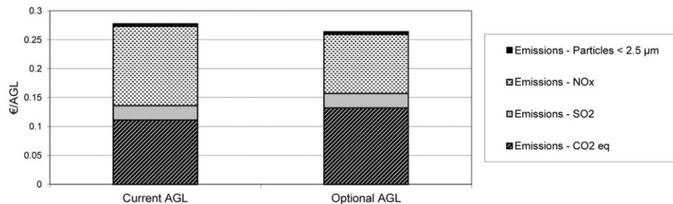
Fig. 6. External costs due to emission of the two AGL systems.
