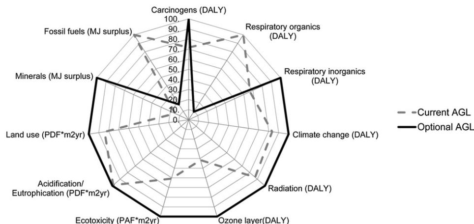
Fig. 2. LCIA characterization results of the two AGL systems, using the EI99 method (adapted from Simões et al., 2010). DALY: Disability Adjusted Life Years (years of disabled living or years of life lost due to the impacts); PAF: Potentially Affected Fraction (animals affected by the impacts); PDF: Potentially Disappeared Fraction (plant species that disappear as result of the impacts); MJ surplus: Surplus Energy (MJ) (extra energy that future generations must use to extract scarce resources).
