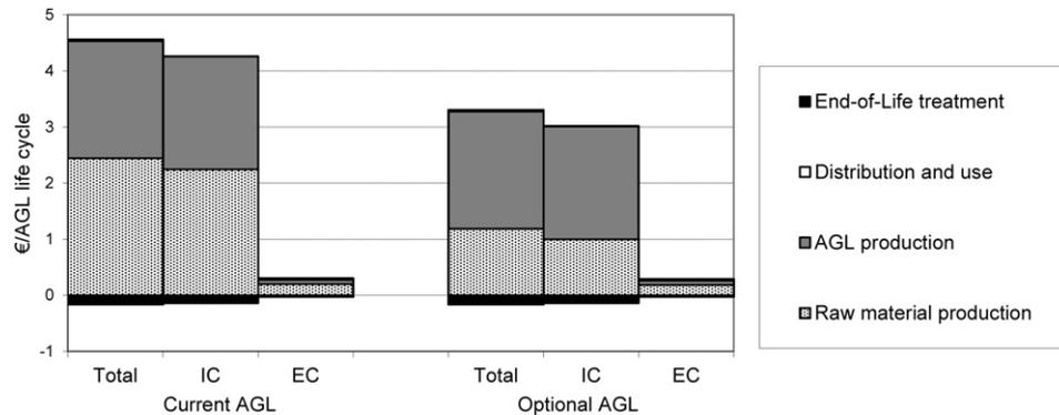
Fig. 5. Internal (IC), external (EC) and total costs of the two AGL systems.
